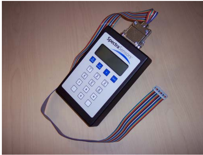
Figure 3: Service Interface Module for Local Test and Evaluation of the SEB
