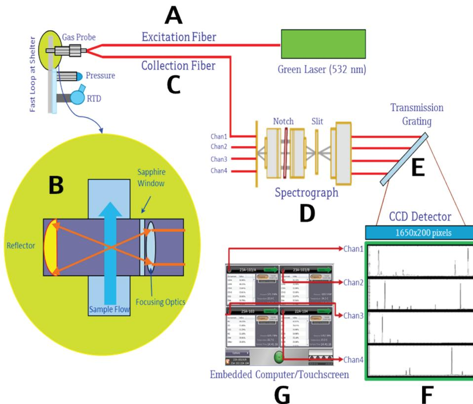
Figure 7. Components of the process Raman analyzer
