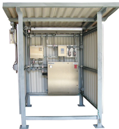
Gas analysis shelter with a TDLAS analyzer mounted inside a three-sided shelter equipped with a fluorescent light, power distribution box, and sample line heat trace controller.
