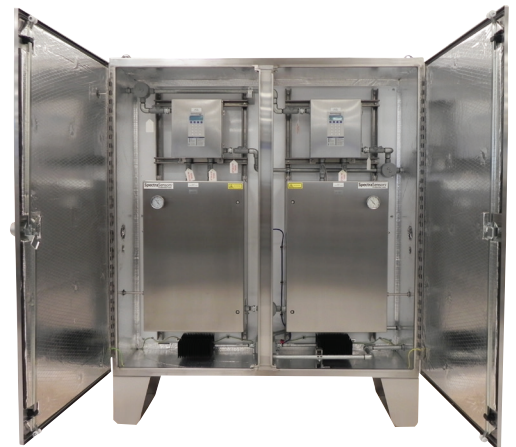
Gas analysis shelter with two TDLAS analyzers inside a heated/insulated cabinet for operation in a cold weather environment.
